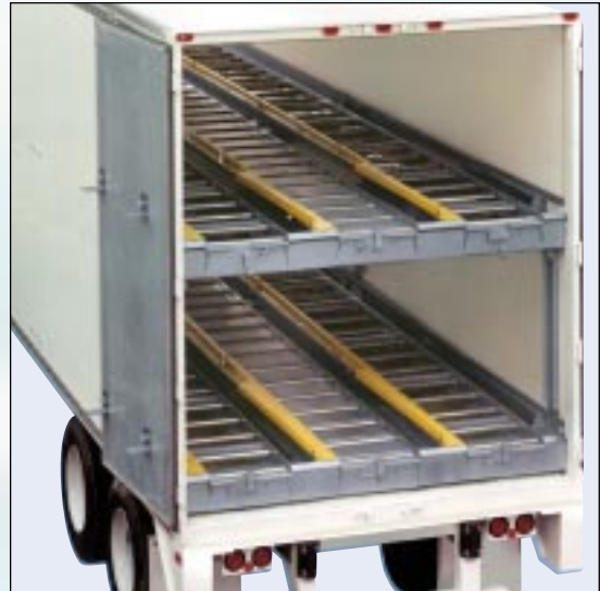
Power-Pack trailer-mounted powered conveyors are ideal solutions for Just-in-Time delivery to line set.
